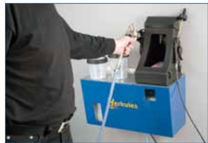
Spray out the remaining paint
