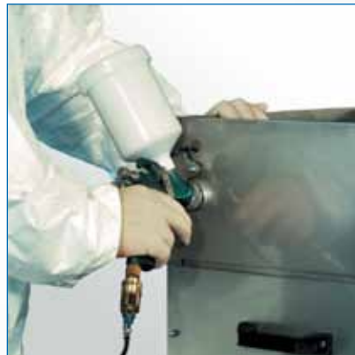
Spray guns and paint cups are simply placed in the drip openings.
