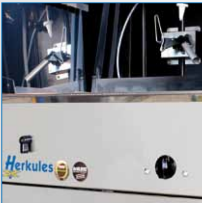
A knob manages the automatic cleaning.
