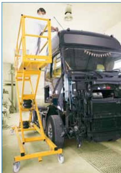
The painter is easily moveable with the wheels. Both at prep work and spray booths – excellent for small spaces.
