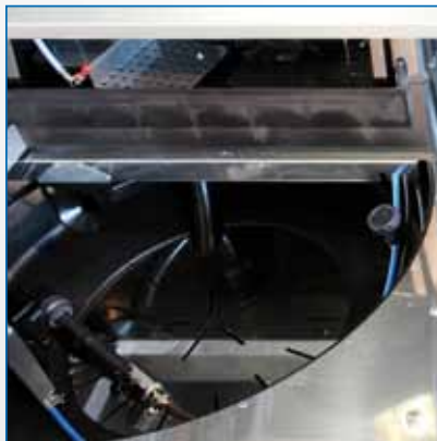
The manual workstation is equipped with brush for re-circulating solvent and a spray gun for fresh solvent.
