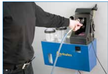
Rinse the paint channel
