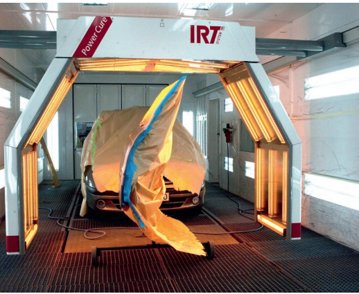
The vehicle and loose parts can be cured in the same drying cycle thanks to the intelligent software technology.
