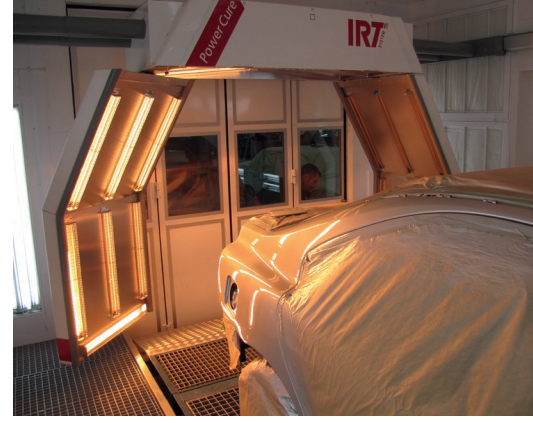
The front and the back of the vehicle are easily cured as the wings can be angled towards the painted surface.
