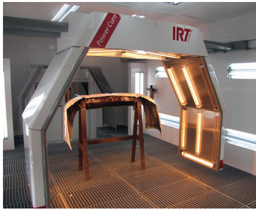
Loose parts are easy to cure. The IRT PowerCure detects the starting position and saves energy by only activating the necessary IR lamps.
