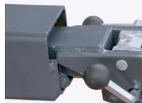
SC (Sports car arms): extremely flat construction. Very sturdy, made of solid material. Especially suitable for very low and wide sports cars.
