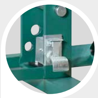
Foot operated air approach feature.
